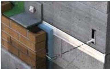
ST-4 Brick relief angle at concrete beam.
